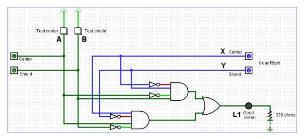
On the summary page, the above circuit is shown combined with two others that are based on analogous Logic Friday expressions for the two fault LEDs, and without additional simplification.
